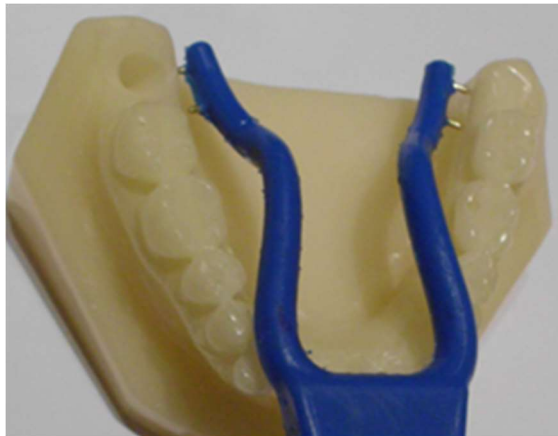
Figure 2 - An upper view of SaliPen proper positioning, with the electrodes placed lingually to the mandibular third molar, which may be either absent (right) or present (left).
